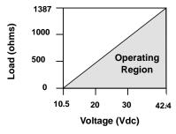
The Field communicator requires a minimum loop resistance of 250 $\Omega$  for communication.
